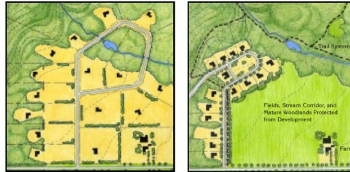
A comparison of a conventional subdivision (left) with a conservation subdivision (right). In both cases, a total of 16 residential lots were created. A conservation easement ensures that the open land preserved as part of the conservation subdivision (right) cannot be further subdivided or developed in the future. Source: Conservation Design for Subdivisions: A Practical Guide to Creating Open Space Networks (1996) by Randall Arendt.
